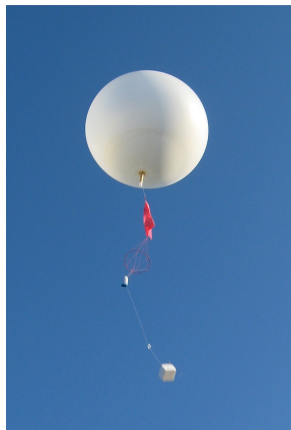
Figure 2. Typical rawinsonde balloon.
