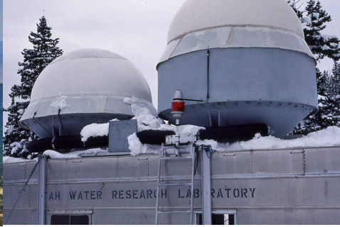
Special radar for detecting small cloud and precipitation particles above Grand Mesa
