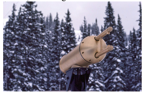
2D-C instrument on a post at Grand Mesa. The laser beam passes between the tips to record shadows of snow.
