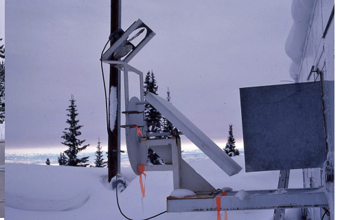
Antenna outside trailer for a microwave radiometer instrument that measures total water vapor and liquid water above Grand Mesa
