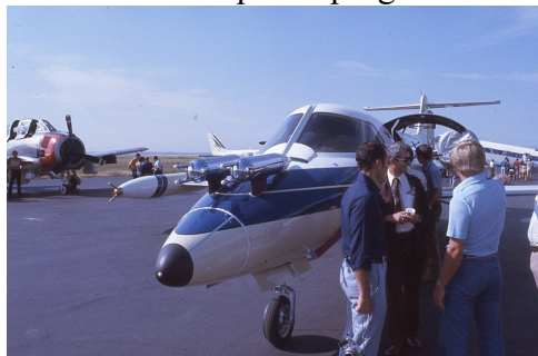
Armor-plated aircraft at left for flying in hail. Several cloud and precipitation particle instruments on LearJet nose and wing tip. Other aircraft in rear.
