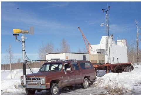
Truck-mounted 2D-C to detect seeded snow crystals passing over highway
