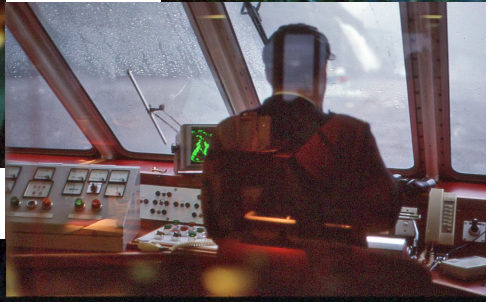
The green radar display guides boat pilot in fog by showing the fjord walls.
