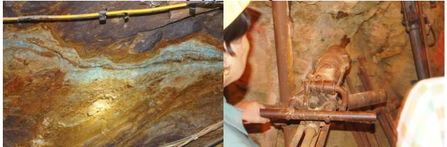
The bluish color is from a copper mineral in the Resurrection Vein inside the mine. The richest gold concentration is the brown in the middle of the blue bands. The equipment scene shows an old drill used to make holes in the rock for insertion of dynamite. It is called the "widow-maker" because it created so much dust that the operators died of lung disease in a few months. Later injections of water in the drilling operation reduced the dust problem.
