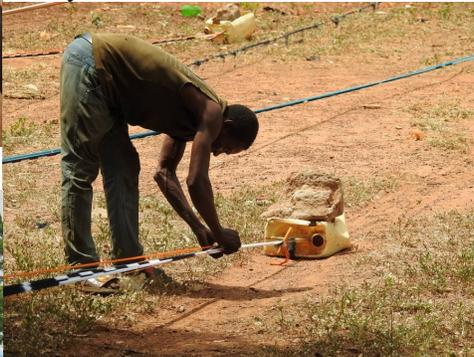
adjusting warp near sliding tension
